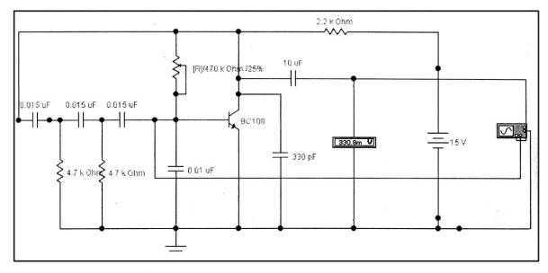
Circuit diagram of RC-Phase Shift Oscillator
