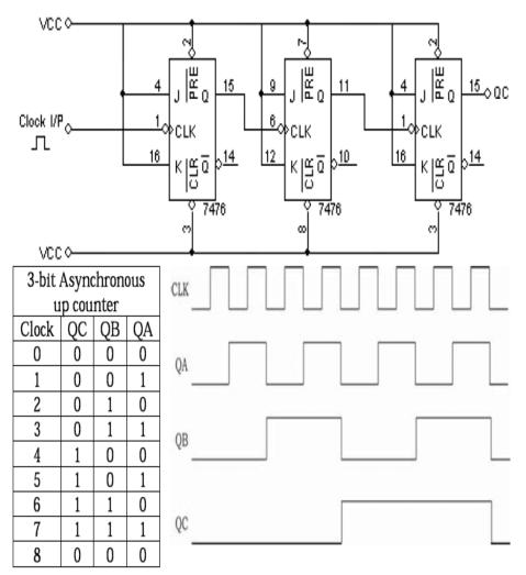
Circuit Diagram: - 3-Bit Asynchronous Up Counter
