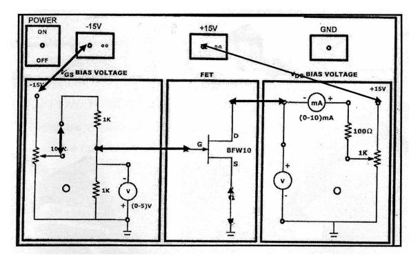
Fig 3.1 WIRING DIAGRAM FET CHARACTERISTICS
